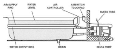
To comply with health regulations and to prevent stagnant water from forming in the system, the bath pump must drain fully after **EVERY** use.
