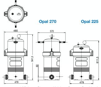
\* Minimum Clearance Height to Remove Cartridge (mm)
