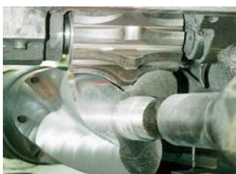
● Rotor processing using a milling machine
