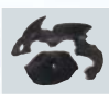
Impeller made of ABS resin After 24 hours of operation Loss of weight: 46%
