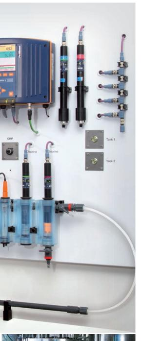
Online process measurement stations are fully assembled and quickly started up. They are central components of control circuits for metering chemicals. The measured values are available in real time around the clock: this applies equally to the efficient control of chemical parameters in process water and determining the quality of treated water.
