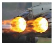
**Titanium: the right stuff for high temperatures** You'll find titanium in military jet engine afterburners.<sup>1</sup>
