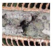
**Rough conditions** High operating temperatures and pool water chemistry can be rough on conventional heat exchanger materials.
