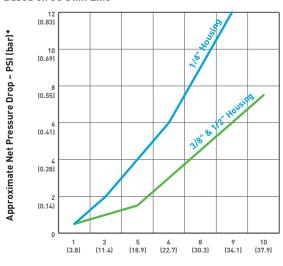
Flow Rate - gpm (lpm)\*
