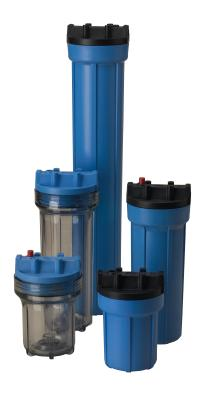
Pentair Slim Line<sup>§</sup> Filter Housings are available in either reinforced polypropylene or clear Styrene-Acrylonitrile (SAN) in 5", 10" and 20" lengths. The black or blue reinforced polypropylene housing caps are available with 1/4", 3/8" or 1/2" NPT connections. Four bosses are molded into every cap for mounting purposes.
