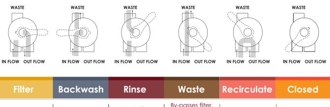
By-passes filter, Used after used for vacuuming Cleaning Filter By-passes filter Shuts off all flow backwash to Normal Filtration by reversing the to waste outlet for circulating flush dirt from to filter or pool flow or lowering water water to pool valve level
