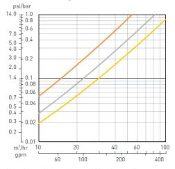
\*head loss is based on a 130 micron disc
