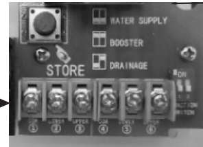
Control terminals for electrical connection to the probe /float switch/pressure switch
