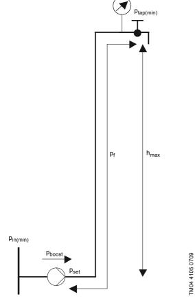
Fig. 9 Calculation of required discharge pressure
