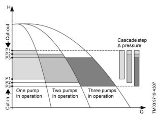
Fig. 2 Operation with cut-in and cut-out
