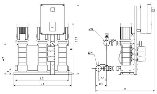
Fig. 13 Dimensional sketch of a Hydro Multi-S booster system with CMV pumps
