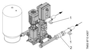
Fig. 8 Example of installation with expansion joints and pipe supports (Grundfos standard scope of supply in grey colour)
