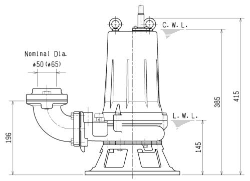
C.W.L.:Continuous running Water Level L.W.L.:Lowest running Water Level
